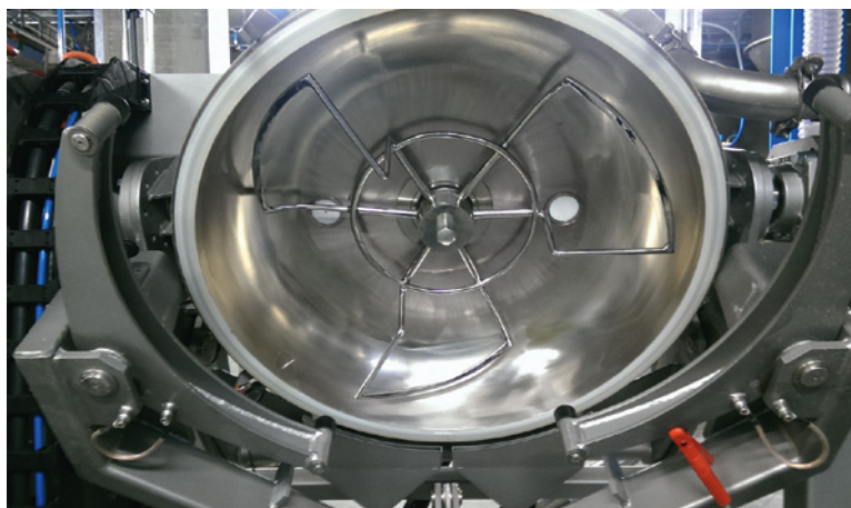
Below: The multiple round bar-profile tool in Henschel's mixer is said to provide high mix quality in vertical mixing positions
