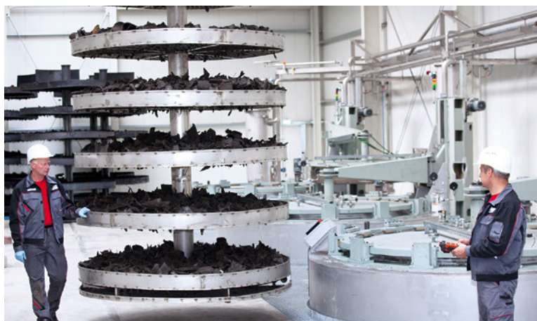
Below: Batch production of carbon black by pyrolysis of used car tyres at Pyrolyx in the Netherlands
